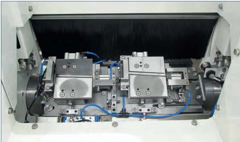
Example pneumatic clamping fixture for package clamping
